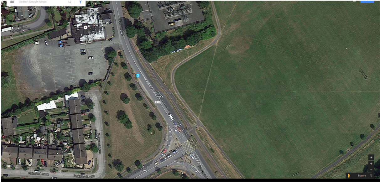
Fig. 5. An aerial view of the proposed development site for the car-park and road access. The proposal is to enter the park at a safe distance from the entrance to the pub car-park to the west of the Old Bawn road and at a safe distance from the road junction shown to the bottom of this image. (Source of this image: Screenshot from Googlemaps 2015)
