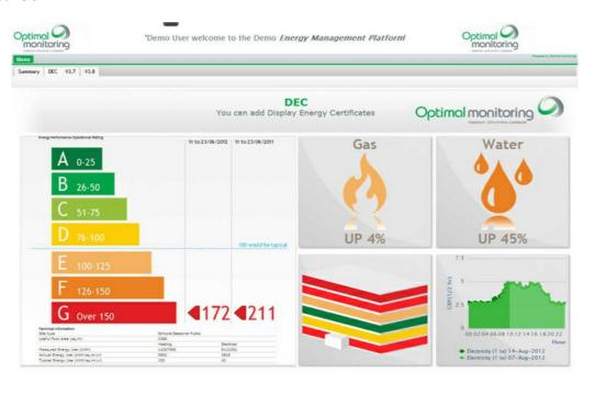
Image 7 - Sample Dashboard Image from a BEMS
